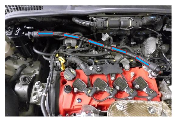
13. The remaining hose is to be fitted to the OUT-PUT of the catch tank, with the hose clamp end going to the intake pipe. Use a 7mm socket or flat blade screwdriver to secure the camp.
