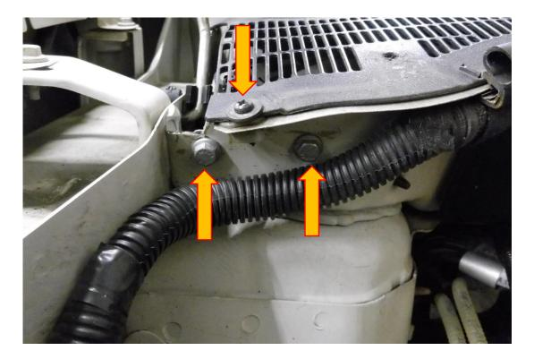
7. Take the catch tank bracket from the kit and using M6 fasteners removed in the previous step mount it to the bulkhead. You will have to hold the sensor behind the bulkhead when re fitting these fasteners. Re fit the Pozi drive fastener.
