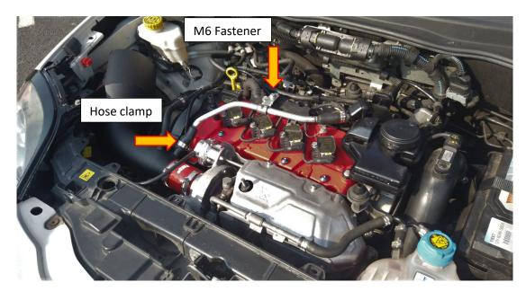
3. Using the 10mm socket and rachet remove the three M6 fasteners attaching the remaining part of the breather system. Finally unclip the hose clamp attaching the hose going to the inlet manifold.
