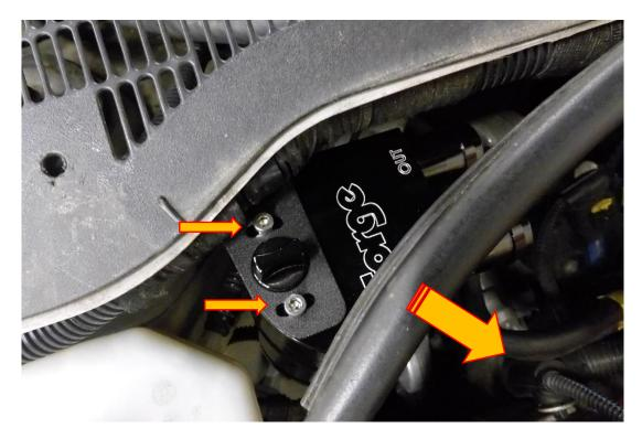
10. Take the machined breather adaptor and retaining bracket from the kit, use the original M6 fastener removed in step 3.
