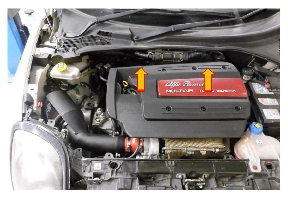
2. Locate the breather system and use a 10mm socket to undo the M6 fastener and a flat blade screwdriver to release the hose clamp attaching the breather to the intake pipe.
