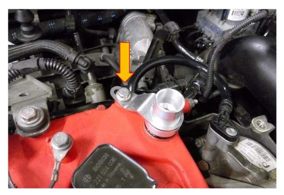
11. Using a 7mm socket and rachet secure the silicone blank to the redundant spout on the inlet manifold.
