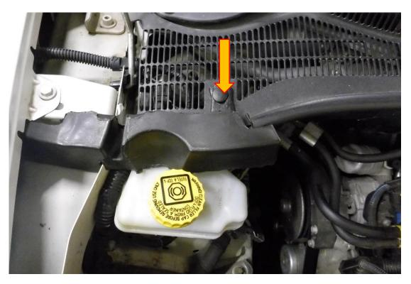
5. Using a flat blade screwdriver push the retaining clip inwards while holding the brake fluid reservoir, then slide it out to the righthand side. (If you have a LHD vehicle you can skip this step.)
