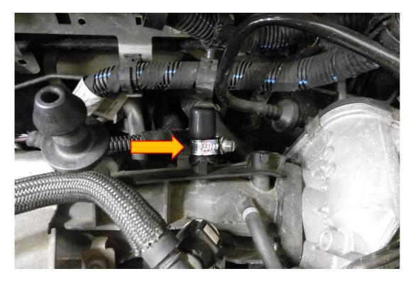
12. Take the larger hose from the kit and fit the 90-degree Norma fitting to the breather adaptor. The other end of the hose needs to be fitted to the IN-PUT of the catch tank.
